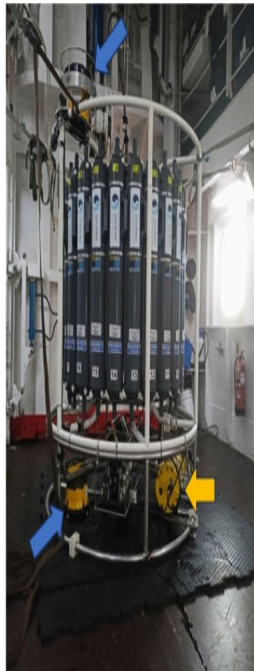
Figure 9. Locations (blue arrows) of the upward and downward looking ADCPs installed in the CTD-rosette ensemble. The external battery canister is marked with an orange arrow.
