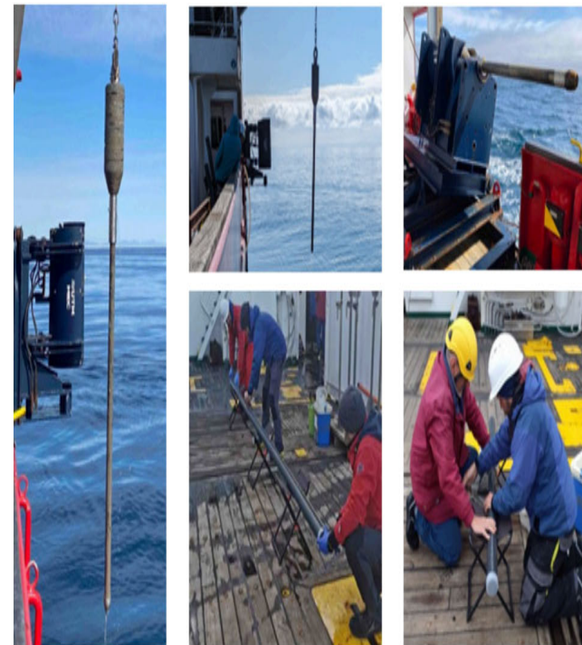
Figure 26. Gravity corer system during the FARDWO-DS1 cruise. Example of a 5 m sediment core recovering, labelling and cutting in 1 m long sections.
