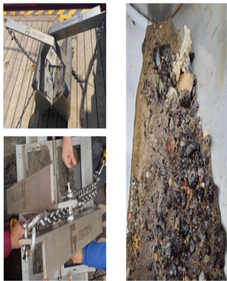
Figure 24. Examples of Van Veen grab recovery with muddy sediments (FDDS1_043_VVb) and a mixture of mud with pebbles (FDDS1_020_VVb).
