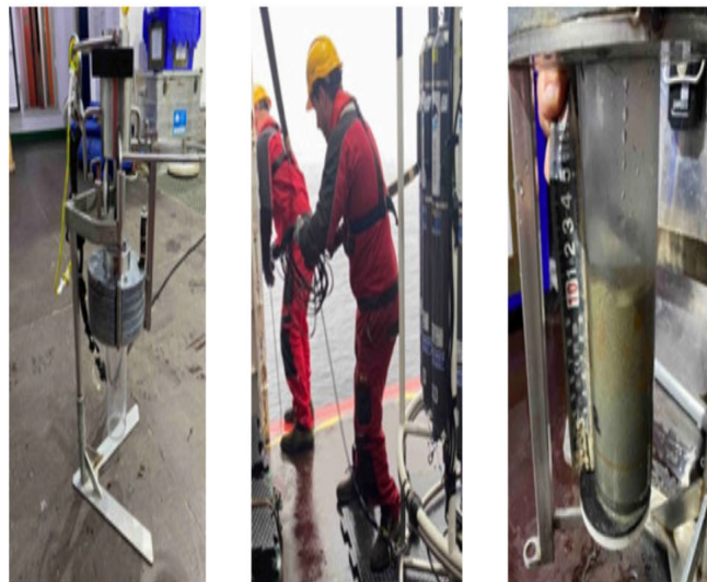
Figure 22. Monocoler system, deployment operation and sample recovered in FDDS1_009_MoC station.
