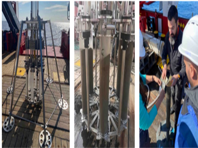
Figure 25. Multicorer system used during FARDWO-DS1 cruise and an example of sediment recovery and sampling.
