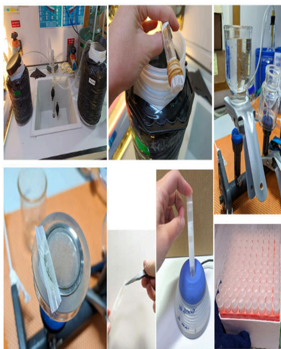
Figure 20. Details of the different steps of the microanalysis sampling.
